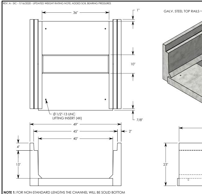
MAX AASHTO H-40 RATED - 64,000 LB. SINGLE AXLE LOAD DEPENDENT ON TRENCH COVER RATING MINIMUM ALLOWABLE SOIL BEARING PRESSURE – H-40: 3,000 PSF; H-20: 3,000 PSF **DESCRIPTION:**
