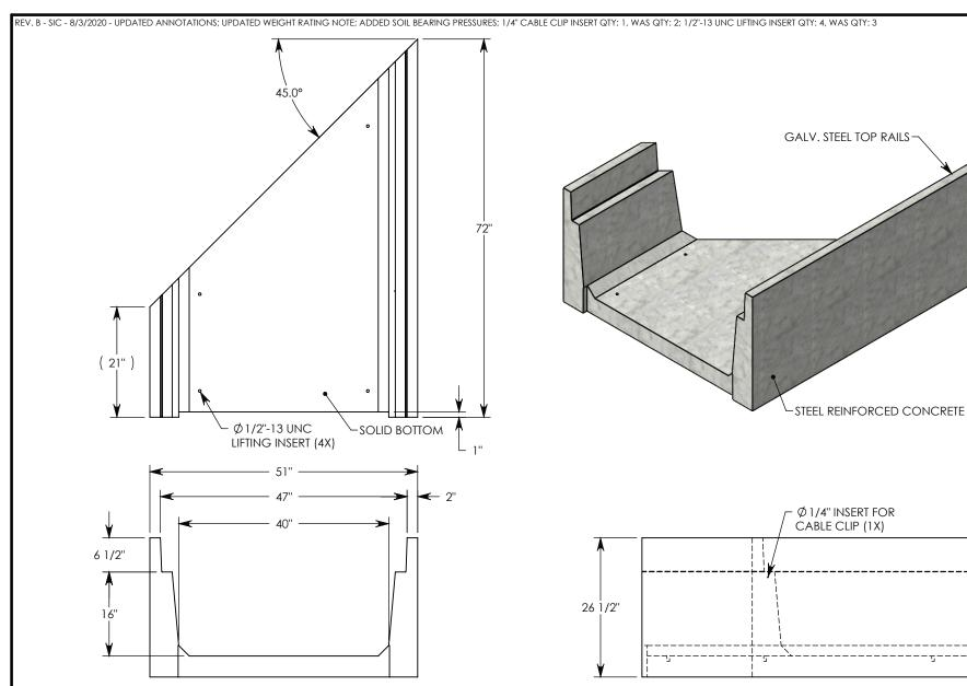
AASHTO H-20 RATED - 32,000 LB. SINGLE AXLE LOAD MINIMUM ALLOWABLE SOIL BEARING PRESSURE – 3,000 PSF
