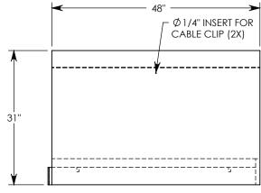
**NOTE 1:** FOR NON-STANDARD LENGTHS THE CHANNEL WILL BE SOLID BOTTOM AND DESIGNATED WITH ITS CORRESPONDING LENGTH MEASUREMENT. IE: 804024HT4 32"
