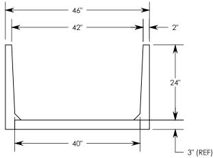
**NOTE:** FOR NON-STANDARD LENGTHS THE CHANNEL WILL BE SOLID BOTTOM AND DESIGNATED WITH ITS CORRESPONDING LENGTH MEASUREMENT. IE: 804024PT 32"
