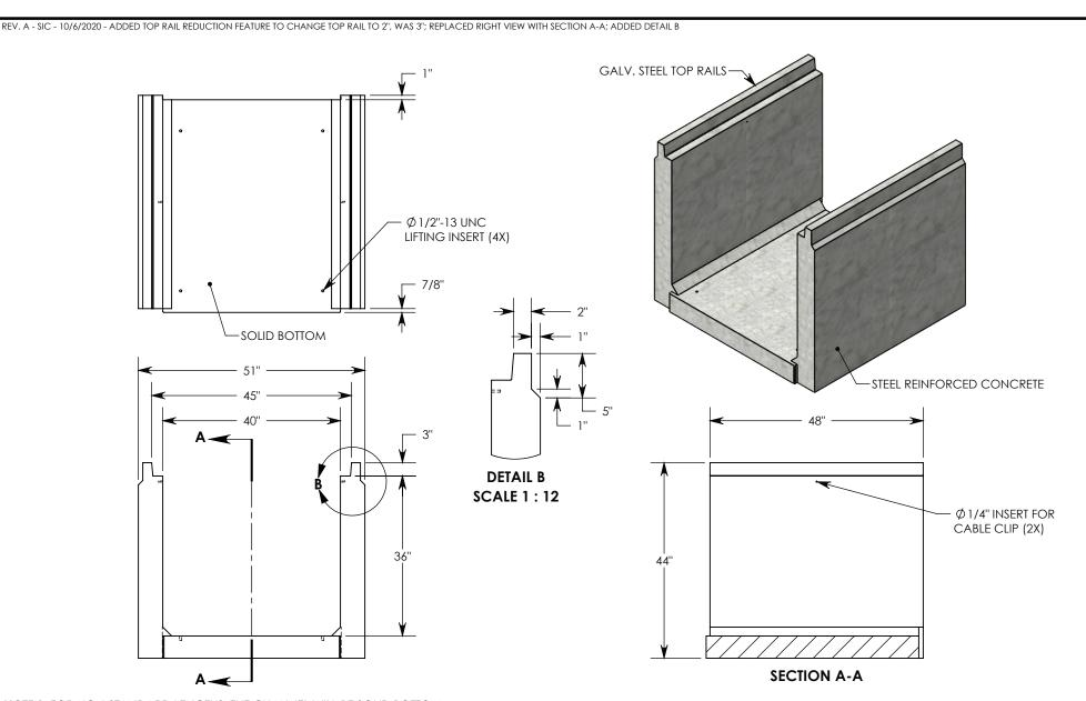
**NOTE 1:** FOR NON-STANDARD LENGTHS, THE CHANNEL WILL BE SOLID BOTTOM AND DESIGNATED WITH ITS CORRESPONDING LENGTH MEASUREMENT. IE: 804036HT3 32"
