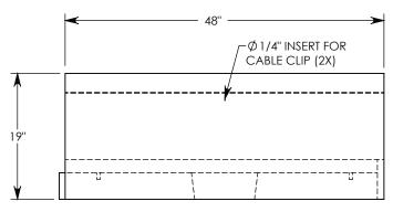
**NOTE 1:** FOR NON-STANDARD LENGTHS, THE CHANNEL WILL BE SOLID BOTTOM AND DESIGNATED WITH ITS CORRESPONDING LENGTH MEASUREMENT. IE: 8040HT3 32"
