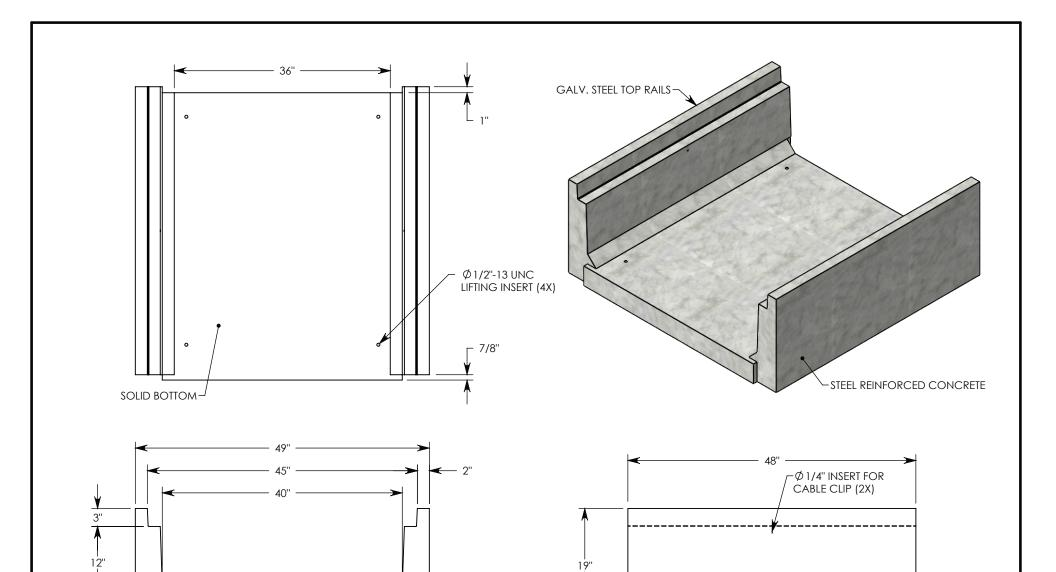
NOTE 1: FOR NON-STANDARD LENGTHS THE CHANNEL WILL BE SOLID BOTTOM & DESIGNATED WITH ITS CORRESPONDING LENGTH MEASUREMENT. IE:8020HT3 32"
