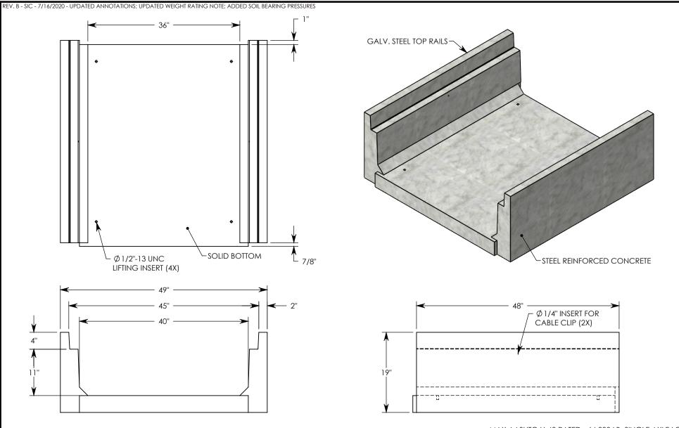
**NOTE 1:** FOR NON-STANDARD LENGTHS THE CHANNEL WILL BE SOLID BOTTOM AND DESIGNATED WITH ITS CORRESPONDING LENGTH MEASUREMENT. IE:8020HT4 32"
