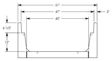
NOTE 1: FOR NON-STANDARD LENGTHS THE CHANNEL WILL BE SOLID BOTTOM AND DESIGNATED WITH ITS CORRESPONDING LENGTH MEASUREMENT. IE: 8040HT 32"
