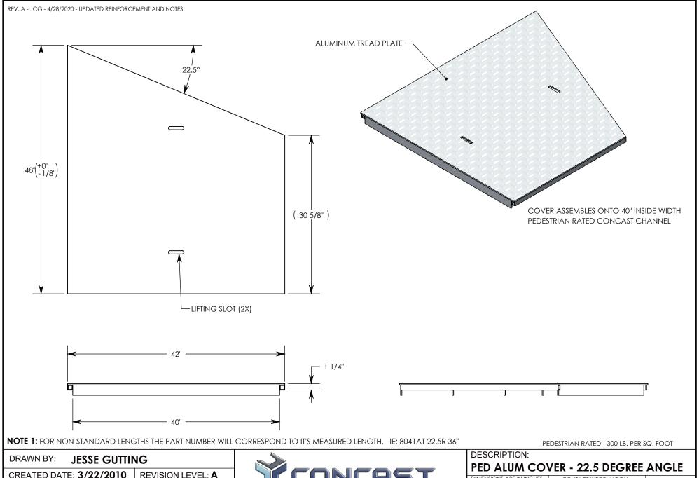
CREATED DATE: 3/22/2010 REVISION LEVEL: A SAVED DATE: 4/28/2020 SAVED BY: jgutting WEIGHT: MATERIAL: **WELDED ALUMINUM** 56 LBS.
