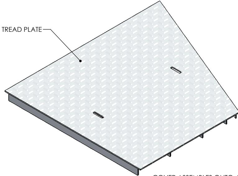
COVER ASSEMBLES ONTO 40" INSIDE WIDTH PEDESTRIAN RATED CONCAST CHANNEL
