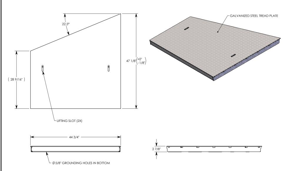
NOTE 1: FOR NON-STANDARD LENGTHS, THE PART NUMBER WILL CORRESPOND TO IT'S MEASURED LENGTH. IE: 8041HTSG 22.5L 18"
