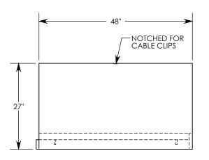
**NOTE:** FOR NON-STANDARD LENGTHS THE CHANNEL WILL BE SOLID BOTTOM AND DESIGNATED WITH ITS CORRESPONDING LENGTH MEASUREMENT. IE: 805024PTSB 32"
