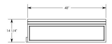
NOTE: FOR NON-STANDARD LENGTHS THE CHANNEL WILL BE SOLID BOTTOM AND DESIGNATED WITH ITS CORRESPONDING LENGTH MEASUREMENT. IE: 8040F 32"
