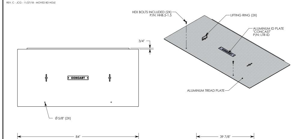
NOTE 1: FOR ADDED SECURITY, PENTA HEAD BOLTS (P/N: PTA.5-1.5) CAN BE ADDED
