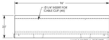
NOTE 1: FOR NON-STANDARD LENGTHS THE CHANNEL WILL BE SOLID BOTTOM AND DESIGNATED WITH ITS CORRESPONDING LENGTH MEASUREMENT. IE: 801016HT3 72" MAX AASHTO H-40 RATED - 64,000 LB. SINGLE AXLE LOAD DEPENDENT ON TRENCH COVER RATING MINIMUM ALLOWABLE SOIL BEARING PRESSURE – H-40: 5,500 PSF; H-20: 3,000 PSF
