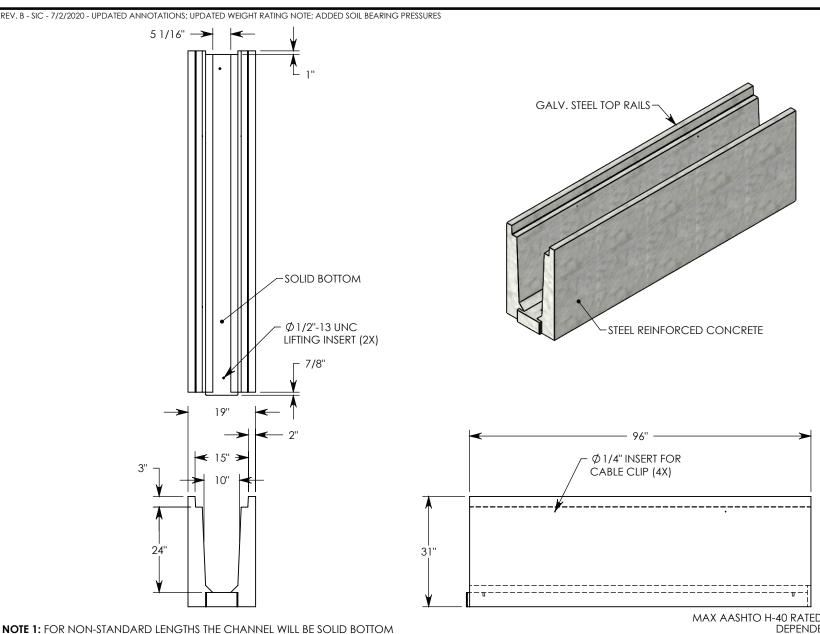
**NOTE 1:** FOR NON-STANDARD LENGTHS THE CHANNEL WILL BE SOLID BOTTOM AND DESIGNATED WITH ITS CORRESPONDING LENGTH MEASUREMENT. IE: 801024HT3 32"
