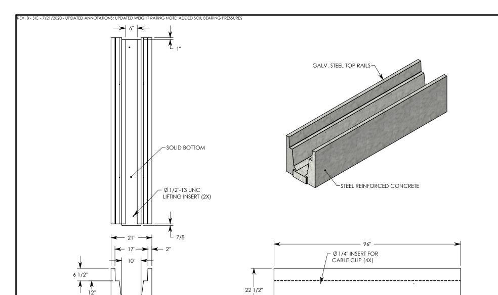
**NOTE 1:** FOR NON-STANDARD LENGTHS THE CHANNEL WILL BE SOLID BOTTOM AND DESIGNATED WITH ITS CORRESPONDING LENGTH MEASUREMENT. IE: 8010HT 32"
