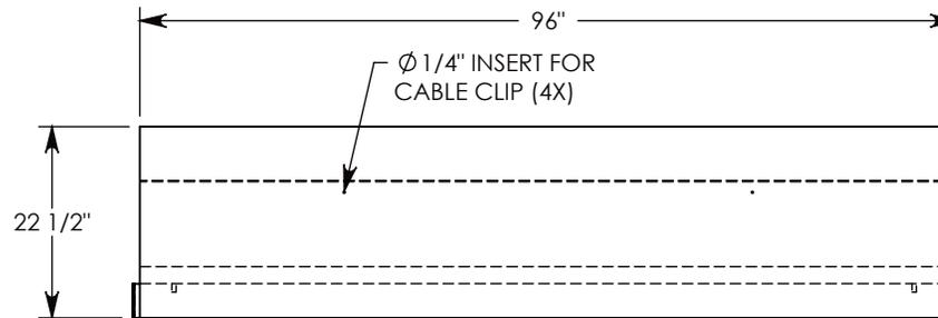
**NOTE 1:** FOR NON-STANDARD LENGTHS THE CHANNEL WILL BE SOLID BOTTOM AND DESIGNATED WITH ITS CORRESPONDING LENGTH MEASUREMENT. IE: 801OHT 32"
