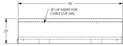
**NOTE 1:** FOR NON-STANDARD LENGTHS THE CHANNEL WILL BE SOLID BOTTOM AND DESIGNATED WITH ITS CORRESPONDING LENGTH MEASUREMENT. IE: 802016HT3 72"
