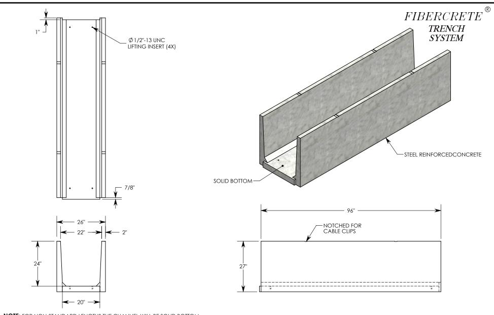
**NOTE:** FOR NON-STANDARD LENGTHS THE CHANNEL WILL BE SOLID BOTTOM AND DESIGNATED WITH ITS CORRESPONDING LENGTH MEASUREMENT. IE: 882024PTSB 32"
