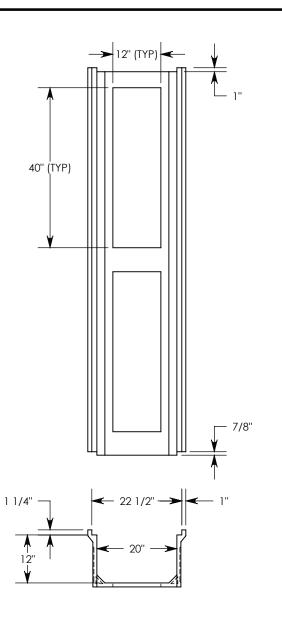
FIBERCRETE® **TRENCH SYSTEM** FIBER & STEEL REINFORCED CONCRETE
