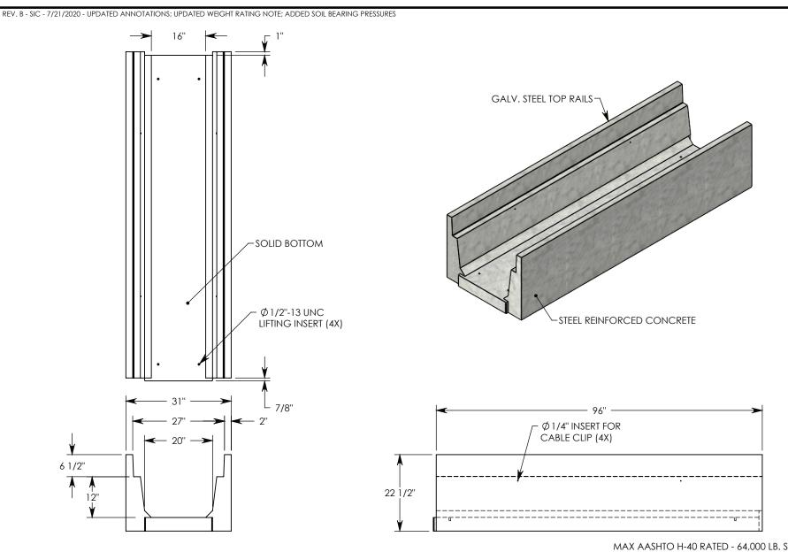
NOTE 1: FOR NON-STANDARD LENGTHS THE CHANNEL WILL BE SOLID BOTTOM AND DESIGNATED WITH ITS CORRESPONDING LENGTH MEASUREMENT. IE: 8020HT 32"
