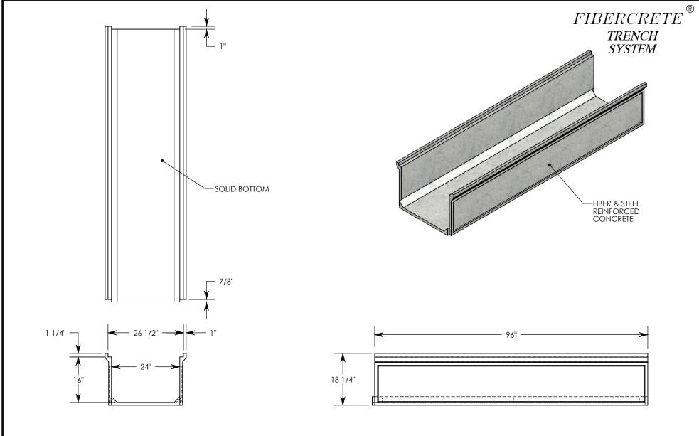
NOTE: FOR NON-STANDARD LENGTHS THE CHANNEL WILL BE DESIGNATED WITH ITS CORRESPONDING LENGTH MEASUREMENT. IE: 882416FSB 32"
