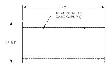
**NOTE 1:** FOR NON-STANDARD LENGTHS THE CHANNEL WILL BE SOLID BOTTOM AND DESIGNATED WITH ITS CORRESPONDING LENGTH MEASUREMENT. IE: 882436HT 36"
