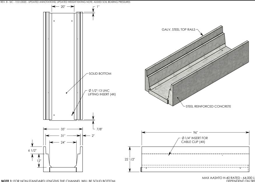
**NOTE 1:** FOR NON-STANDARD LENGTHS THE CHANNEL WILL BE SOLID BOTTOM AND DESIGNATED WITH ITS CORRESPONDING LENGTH MEASUREMENT. IE: 8024HT 32"
