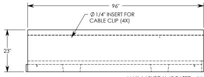
**NOTE 1:** FOR NON-STANDARD LENGTHS THE CHANNEL WILL BE SOLID BOTTOM AND DESIGNATED WITH ITS CORRESPONDING LENGTH MEASUREMENT. IE: 803016HT3 72"
