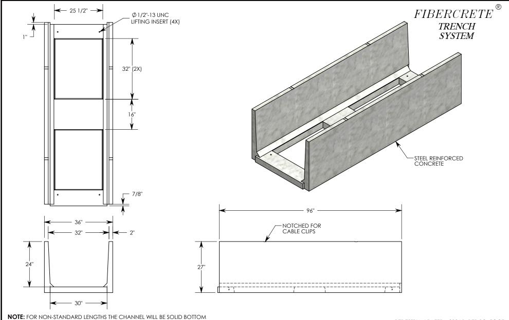
**NOTE:** FOR NON-STANDARD LENGTHS THE CHANNEL WILL BE SOLID BOTTOM AND DESIGNATED WITH ITS CORRESPONDING LENGTH MEASUREMENT. IE: 883024PT 32"
