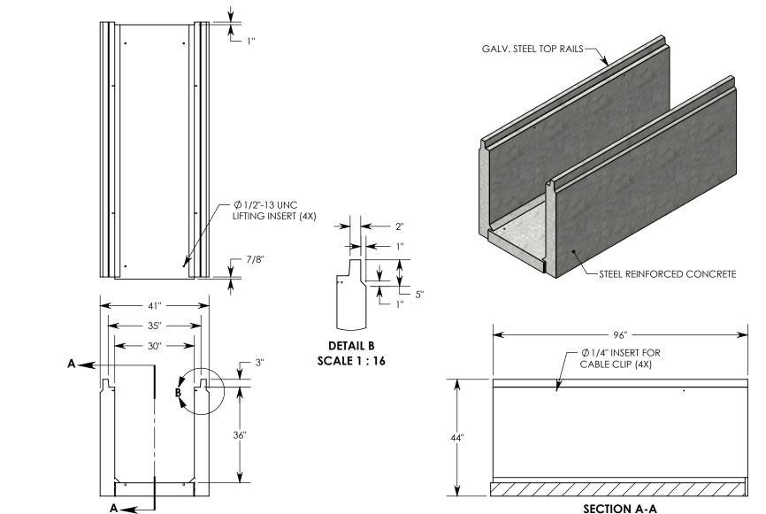
**NOTE 1:** FOR NON-STANDARD LENGTHS, THE CHANNEL WILL BE SOLID BOTTOM AND DESIGNATED WITH ITS CORRESPONDING LENGTH MEASUREMENT. IE: 803036HT3 32"
