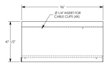
NOTE 1: FOR NON-STANDARD LENGTHS THE CHANNEL WILL BE SOLID BOTTOM AND DESIGNATED WITH ITS CORRESPONDING LENGTH MEASUREMENT. IE: 883036HT 36"
