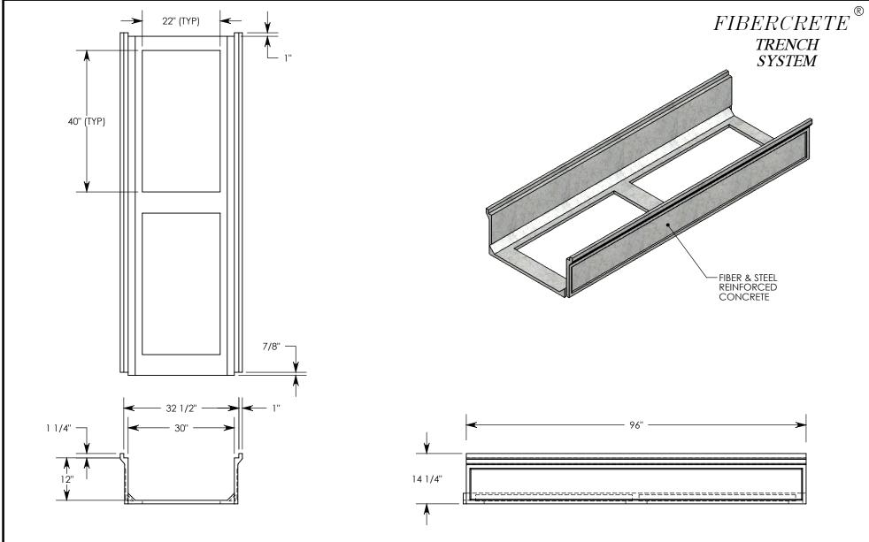
NOTE: FOR NON-STANDARD LENGTHS THE CHANNEL WILL BE SOLID BOTTOM AND DESIGNATED WITH ITS CORRESPONDING LENGTH MEASUREMENT. IE: 8830F 32"
