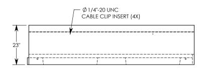
**NOTE 1:** FOR NON-STANDARD LENGTHS THE CHANNEL WILL BE SOLID BOTTOM AND DESIGNATED WITH ITS CORRESPONDING LENGTH MEASUREMENT. IE: 804016LT4 32"
