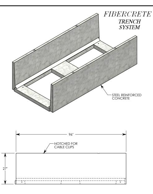
**NOTE:** FOR NON-STANDARD LENGTHS THE CHANNEL WILL BE SOLID BOTTOM AND DESIGNATED WITH ITS CORRESPONDING LENGTH MEASUREMENT. IE: 884024PT 32"
