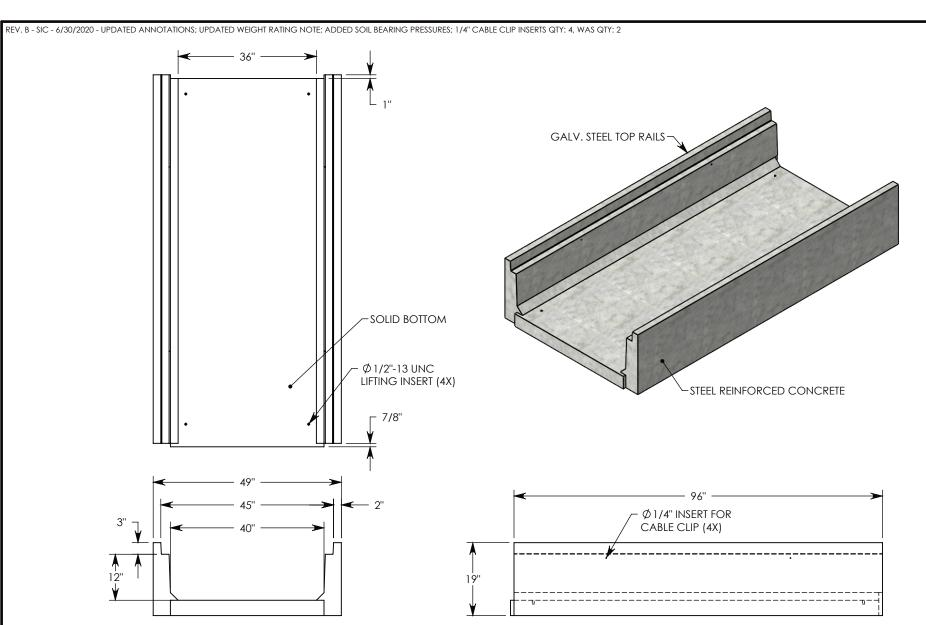
NOTE 1: FOR NON-STANDARD LENGTHS, THE CHANNEL WILL BE SOLID BOTTOM AND DESIGNATED WITH ITS CORRESPONDING LENGTH MEASUREMENT. IE: 8030HT3 72" MAX AASHTO H-40 RATED - 64,000 LB. SINGLE AXLE LOAD DEPENDENT ON TRENCH COVER RATING MINIMUM ALLOWABLE SOIL BEARING PRESSURE – H-40: 3,000 PSF; H-20: 3,000 PSF
