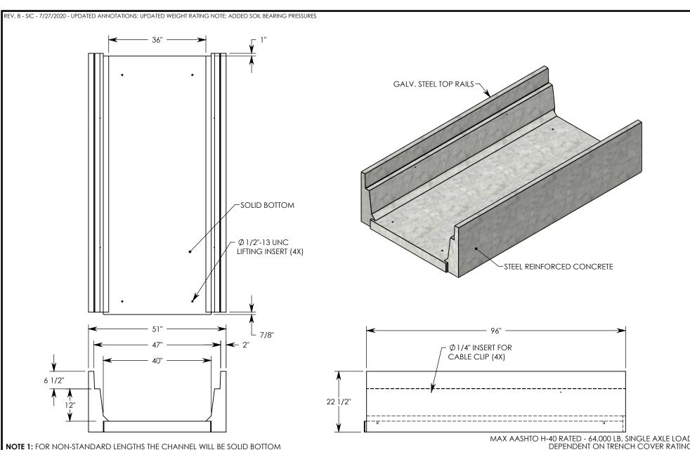
**NOTE 1:** FOR NON-STANDARD LENGTHS THE CHANNEL WILL BE SOLID BOTTOM AND DESIGNATED WITH ITS CORRESPONDING LENGTH MEASUREMENT. IE: 8040HT 32"
