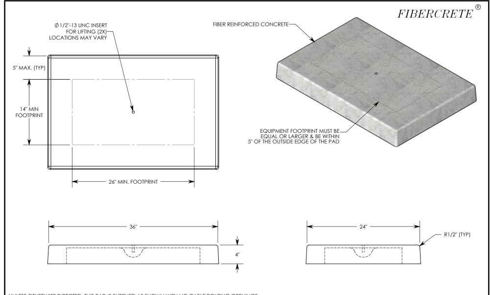
UNLESS OTHERWISE DIRECTED, THIS PAD IS SUPPLIED AS SHOWN WITH NO CABLE ROUTING OPENINGS.
