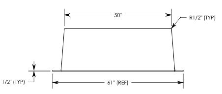
$\phi$  1/2"-13 unc lifting inserts will be cast into box pad if specific inserts or mounting hardware are required, please specify when ordering.
