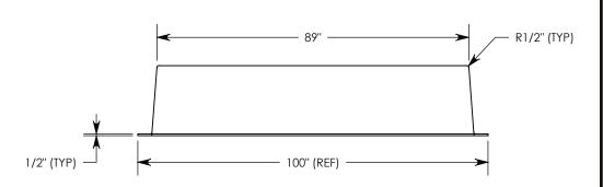
$\phi$  1/2"-13 UNC LIFTING INSERTS WILL BE CAST INTO BOX PAD IF SPECIFIC INSERTS OR MOUNTING HARDWARE ARE REQUIRED, PLEASE SPECIFY WHEN ORDERING.
