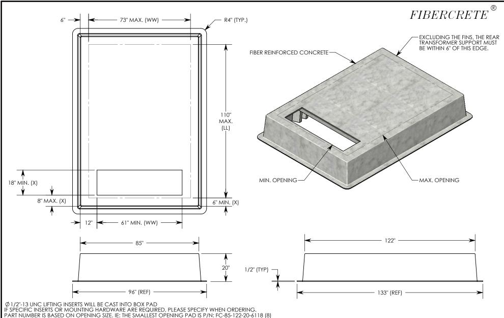
PART NUMBER IS BASED ON OPENING SIZE. IE: THE SMALLEST OPENING PAD IS P/N: FC-85-122-20-6118 (8) THE LARGEST OPENING PAD IS P/N: FC-85-122-20-73110
