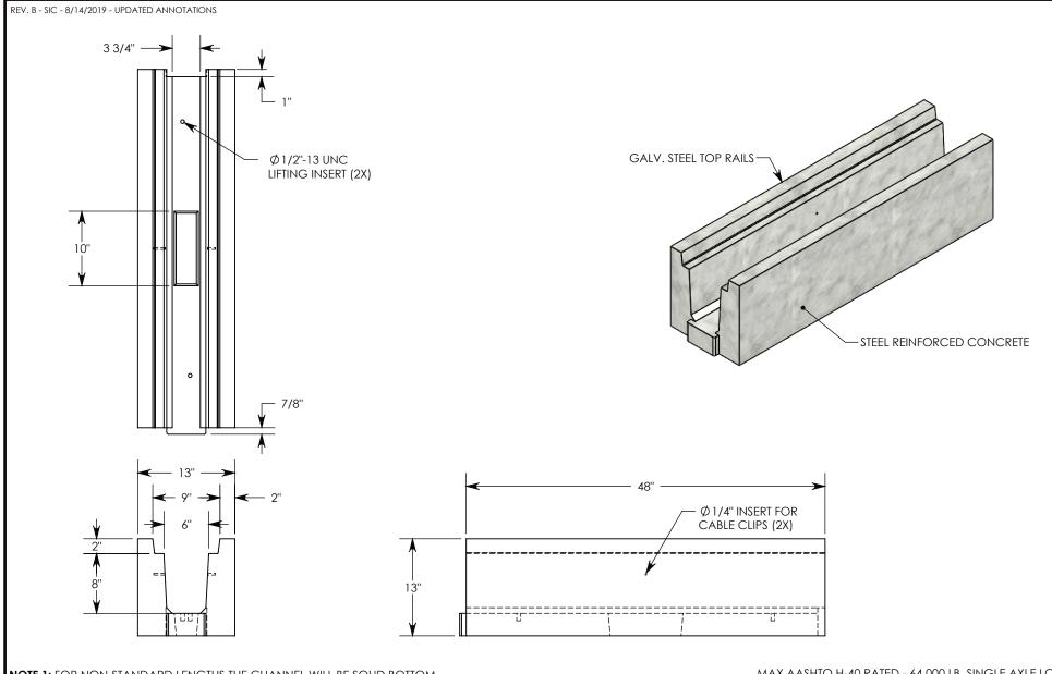
NOTE 1: FOR NON-STANDARD LENGTHS THE CHANNEL WILL BE SOLID BOTTOM AND DESIGNATED WITH ITS CORRESPONDING LENGTH MEASUREMENT. IE: HT0608 32"
