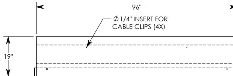
**NOTE 1:** FOR NON-STANDARD LENGTHS THE CHANNEL WILL BE SOLID BOTTOM AND DESIGNATED WITH ITS CORRESPONDING LENGTH MEASUREMENT. IE: HT4F4012 36"
