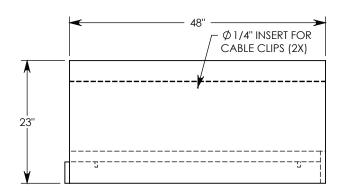
NOTE 1: FOR NON-STANDARD LENGTHS THE CHANNEL WILL BE SOLID BOTTOM AND DESIGNATED WITH ITS CORRESPONDING LENGTH MEASUREMENT. IE: HT4F4016 32" MAX AASHTO H-40 RATED - 64,000 LB. SINGLE AXLE LOAD DEPENDENT ON TRENCH COVER RATING MINIMUM ALLOWABLE SOIL BEARING PRESSURE – H-40: 3,000 PSF; H-20: 3,000 PSF
