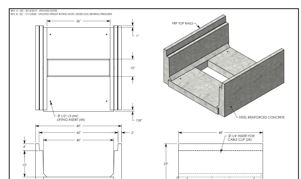
**NOTE 1:** FOR NON-STANDARD LENGTHS THE CHANNEL WILL BE SOLID BOTTOM AND DESIGNATED WITH ITS CORRESPONDING LENGTH MEASUREMENT. IE: HT4F4016 32"
