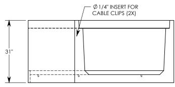
AASHTO H-20 RATED - 32,000 LB. SINGLE AXLE LOAD MINIMUM ALLOWABLE SOIL BEARING PRESSURE – 3,000 PSF
