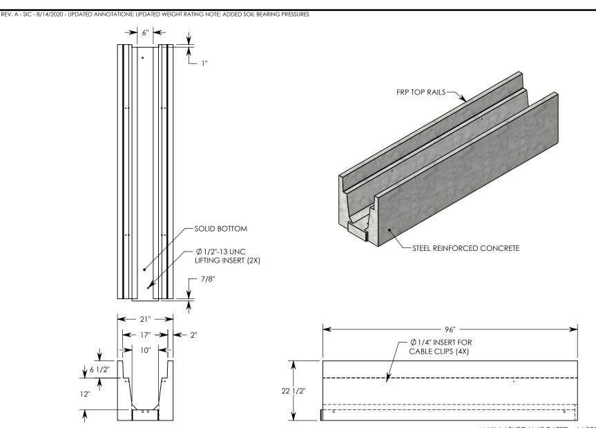
**NOTE 1:** FOR NON-STANDARD LENGTHS THE CHANNEL WILL BE SOLID BOTTOM AND DESIGNATED WITH ITS CORRESPONDING LENGTH MEASUREMENT. IE: HT6F1012 36"
