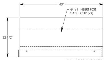
**NOTE 1:** FOR NON-STANDARD LENGTHS THE CHANNEL WILL BE SOLID BOTTOM AND DESIGNATED WITH ITS CORRESPONDING LENGTH MEASUREMENT. IE: HT6F1012 32"
