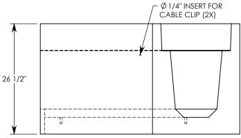
MAX AASHTO H-40 RATED - 64,000 LB. SINGLE AXLE LOAD DEPENDENT ON TRENCH COVER RATING
