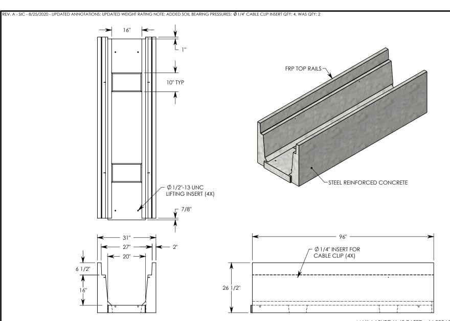
**NOTE 1:** FOR NON-STANDARD LENGTHS THE CHANNEL WILL BE SOLID BOTTOM AND DESIGNATED WITH ITS CORRESPONDING LENGTH MEASUREMENT. IE: HT6F2016 32"
