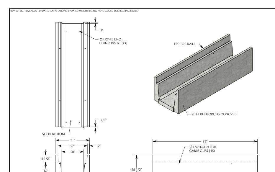
**NOTE 1:** FOR NON-STANDARD LENGTHS THE CHANNEL WILL BE SOLID BOTTOM AND DESIGNATED WITH ITS CORRESPONDING LENGTH MEASUREMENT. IE: HT6F2016 36"
