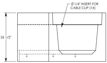
MAX AASHTO H-40 RATED - 64,000 LB. SINGLE AXLE LOAD DEPENDENT ON TRENCH COVER RATING MINIMUM ALLOWABLE SOIL BEARING PRESSURE – H-40: 4,000 PSF; H-20: 3,000 PSF
